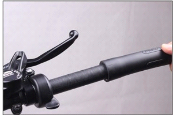
5. fit the new handle bars (left & right; you may need to warm the handle bars if they are hard to fit)
